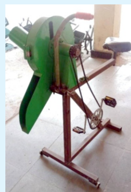
Isometric view of turmeric/ginger slicer
